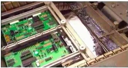
With MB Manufacturing's continuous improvement strategy, we have developed the ultimate selective solder fixture out of a combination of titanium and composite. Incorporating the latest in flow technologies to eliminate skips on bridges. This selective solder pallet will last for years in a high production environment.
